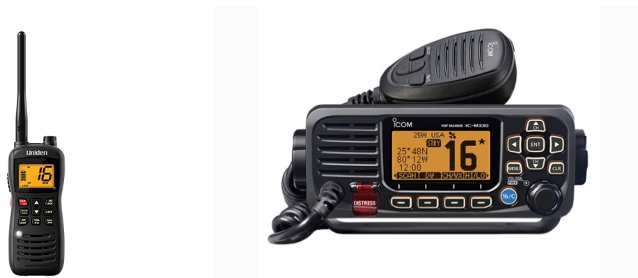
Fig 10.8: Portable and fixed VHF Set
