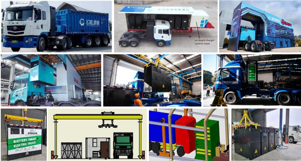
Figure 84 : Battery Swapping Infrastructure for Heavy Trucks
