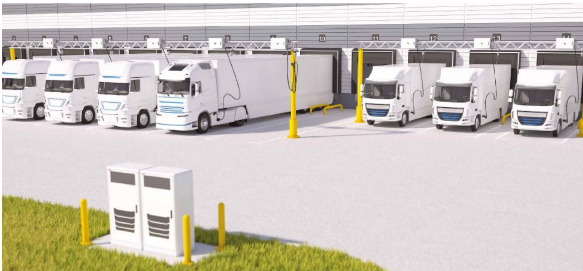
Figure 83 : Drop Cable System of Charging
