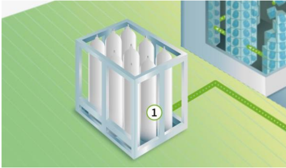
Figure 57 : 1. Source of hydrogen - Low pressure H 2 is stored in bottles ("cylinder racks"), tanks or tube trailers
