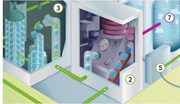
Figure 58 : 2. Boosters - H 2 is compressed using boosters
